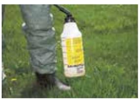
For a quick and reliable reading of the quantity sprayed on the test, use the KALIBOTTLE to calibrate your sprayer. (see calibration table)
